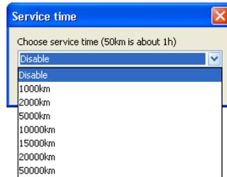
Service time is being signaled only when “*Total working time [hh:mm]*” will reach the value set in “*Service time [hh:mm]*”. When it will exceed that value then after every start of the car in “*Auto mode*” the buzzer will sound for a short period,yellow diode will blink few times and car will automatically go back to “*Petrol mode*”. In such case we need to press button to go back to “*Auto mode*” every time when we want to drive on gas unless we will disable or set another Service inspection.
