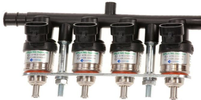
The injectors efficiency should be selected in such way so that at low and high engine load conditions the petrol injection opening time on gas should be equal to petrol injection opening time on petrol. Tables given below should help to make right choice.
