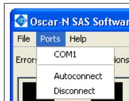
*Autoconnect* function is searching for a controller starting from the lowest COM number found in the system. Therefore it is recommended to assign for connected diagnostic interface the lowest possible COM port index to establish connection more quickly. We can always cancel *Autoconnect* procedure by selecting **“Disconnect”** and select COM port manually.
